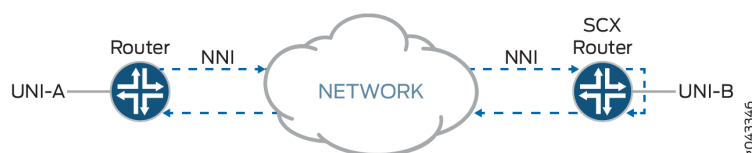
Figure 73: Testing End-to-End Service in Ethernet Loopback Mode
