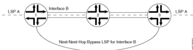
Figure 19: Node Protection Creating a Next-Next-Hop Bypass LSP
