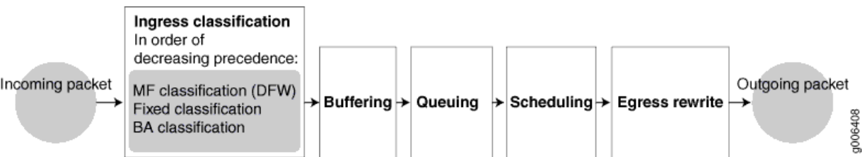
Figure 4: ACX Series Router Packet Forwarding and Data Flow
