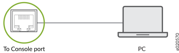
Figure 27: Connect an ACX710 Router Directly to a Management Console
