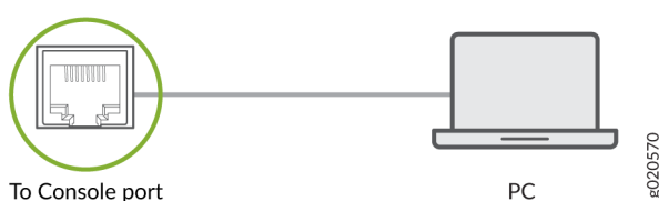
Figure 53: Connecting the ACX7100-32C Router Directly to a Management Console
