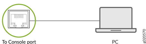
Figure 50: Connect the ACX7348 Router Directly to a Management Console
