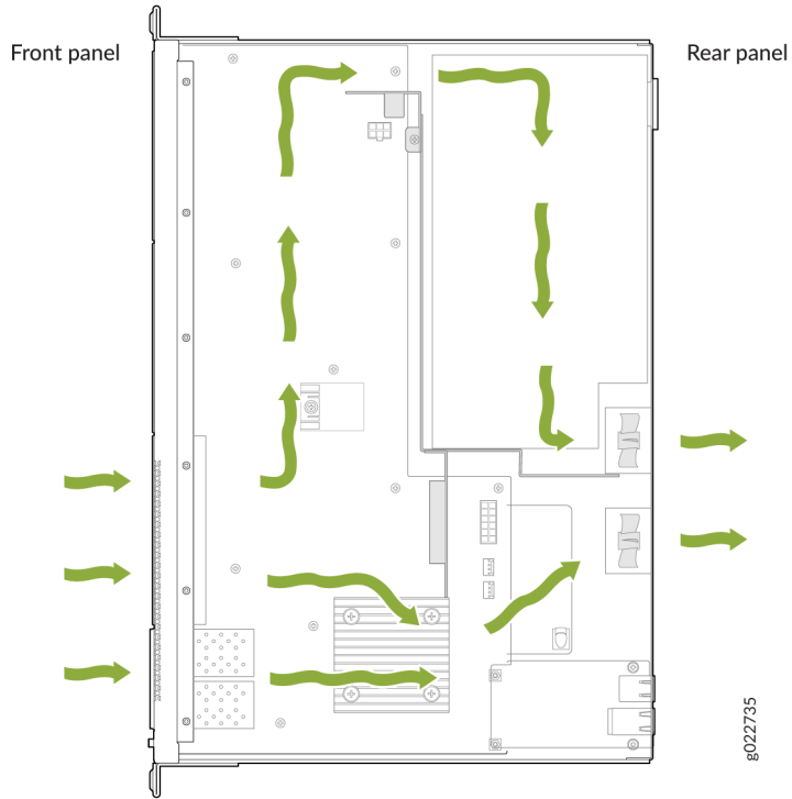
Figure 41: Front-to-Back Airflow Through the EX4100-F-48P Switch Chassis
