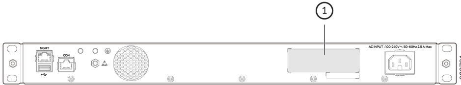
Figure 126: Location of the Serial Number ID Label on the EX4100-F-24T and EX4100-F-48T Switches
