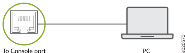
Figure 74: Connect a Device Directly to a Management Console
