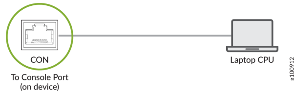
Figure 63: Connect the MX10004 Router Directly to a Management Console
