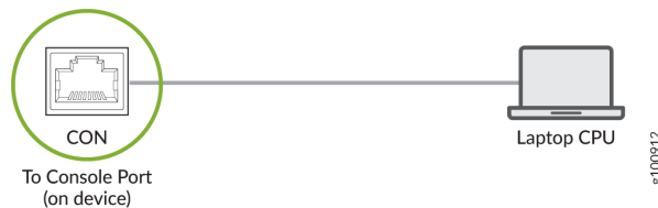
Figure 38: Connecting the NFX350 Device Directly to a Management Console
