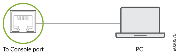
Figure 14: Connect a Device Directly to a Management Console
