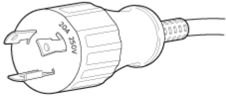
Figure 121: Plug Type for the 20-A Connector
