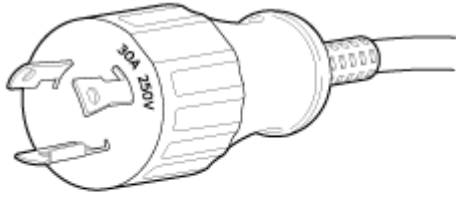
Figure 123: Plug Types for the 30-A Connector
