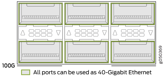
Figure 14: 100-Gigabit Ethernet Ports Are Indicated by a Black Line Underneath the Port
