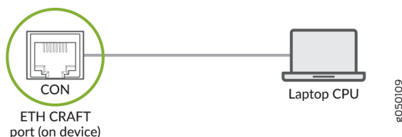
Figure 39: Connecting the QFX Series Directly to a Management Console
