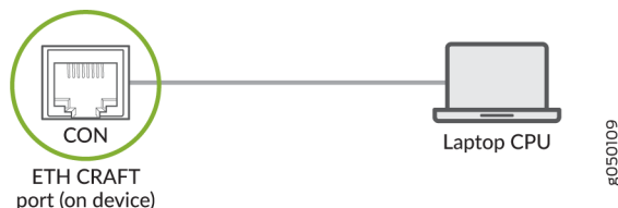
Figure 39: Connecting the QFX Series Directly to a Management Console
