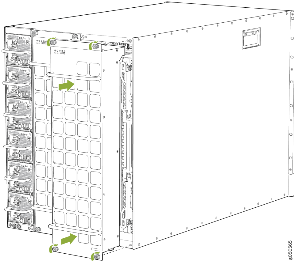
Figure 105: Installing a JNP10008-FAN Fan Tray in a QFX10008 Chassis
