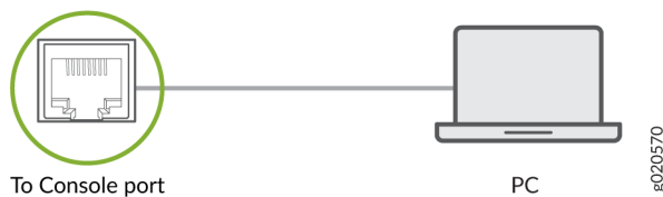
Figure 92: Connect a Device Directly to a Management Console
