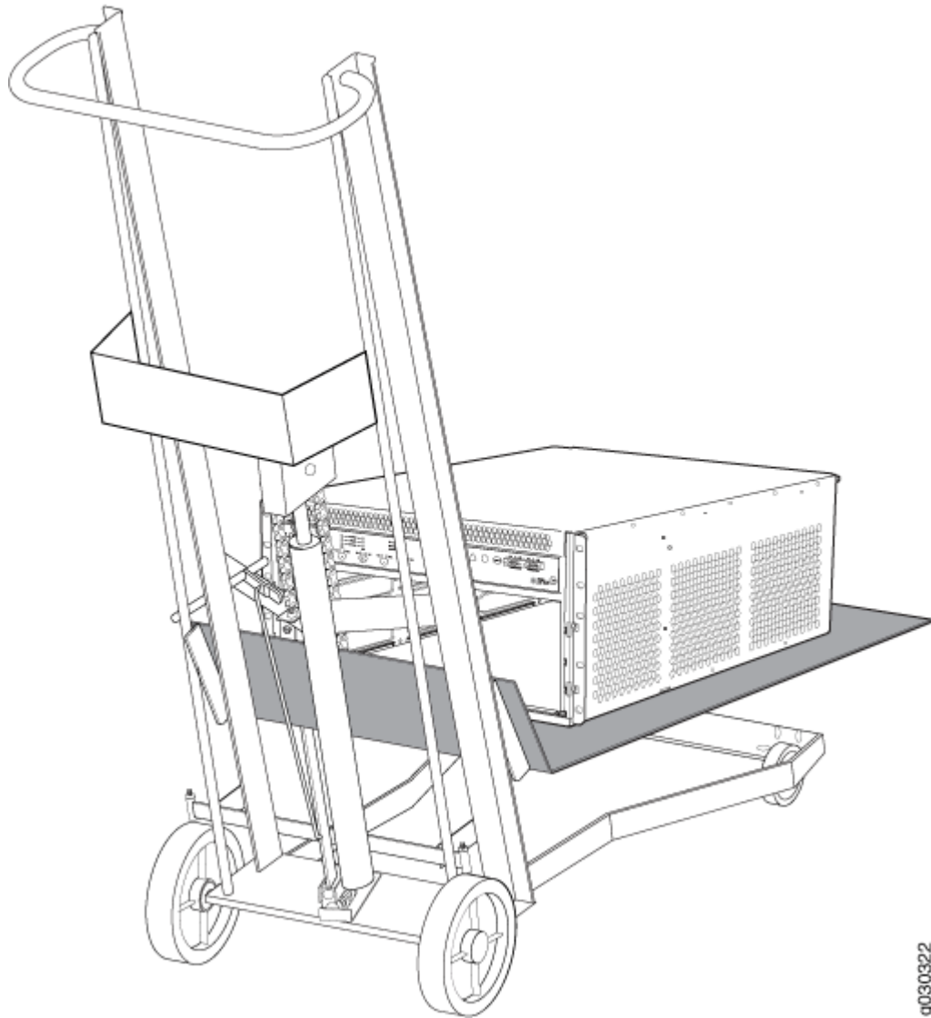
Figure 6: Load the Firewall onto the Lift
