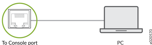
Figure 47: Connecting the Your Device directly to a Management Console
