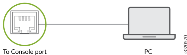
Figure 44: Connecting the Your Device directly to a Management Console
