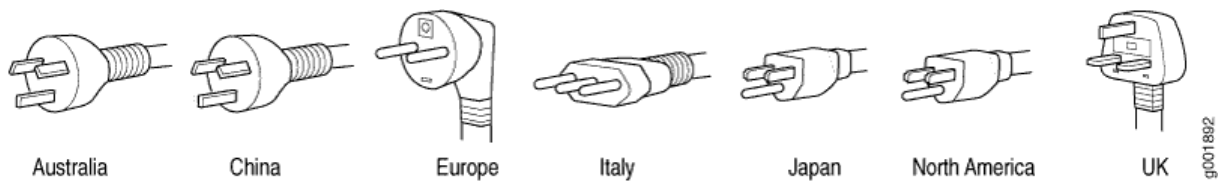
Figure 19: AC Plug Types
