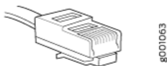
Figure 108: Routing Engine Console and Auxiliary Cable Connector
