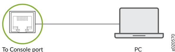
Figure 18: Connecting the SSR1400 directly to a Management Console
