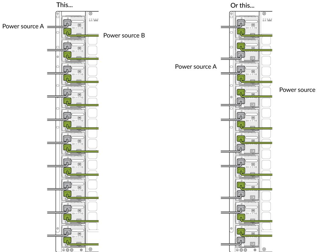
10. Insert the Anderson connector at the end of each power cord into the power supply. The connector snaps and locks the cord into position.
