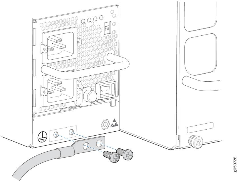
5. Secure the grounding lug to the protective earthing terminal using the screws you removed in step 3.
