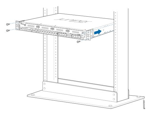
**6.** Check that the mounting brackets on each side of the rack are level.
