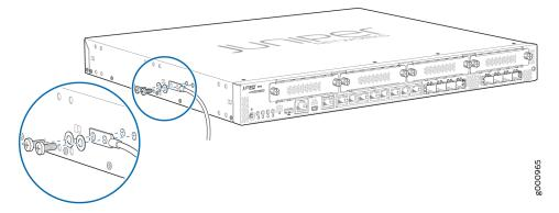
**3.** Plug the power cord into the SRX340 rear panel.
