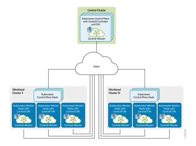
Centralizing the network function in this way makes it not only easier to configure and manage, but also easier to apply consistent network policy and security.
