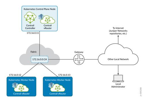
All communication between nodes in the cluster and between nodes and external sites takes place over the single 172.16.0.0/24 fabric virtual network. The fabric network provides the underlay over which the cluster runs.
