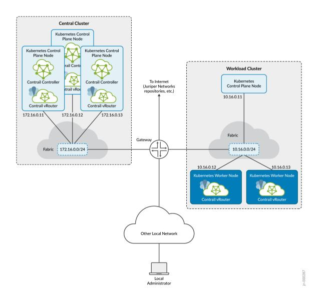
The central cluster attaches to the 172.16.0.0/24 network while the distributed workload cluster attaches to the 10.16.0.0/24 network. A gateway sitting between the networks provides access to each other and external access for downloading images from Juniper Networks repositories.
