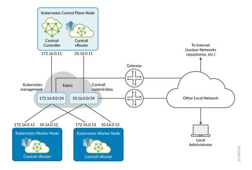
Kubernetes control plane traffic goes over the 172.16.0.0/24 fabric virtual network while Contrail control and data traffic go over the 10.16.0.0/24 fabric virtual network. The fabric networks provide the underlay over which the cluster runs.
