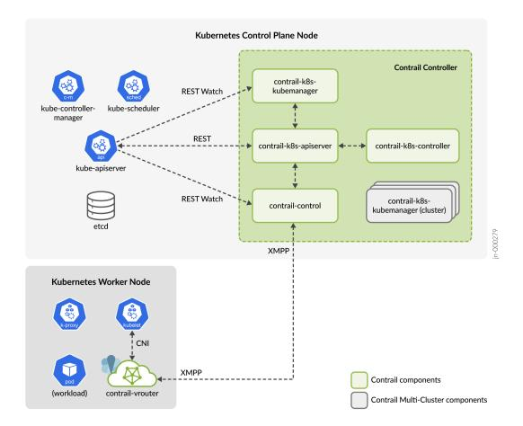
**NOTE**: Starting in release 22.2, Contrail uses its own etcd database by default when running on OpenShift. In earlier releases and in all Contrail releases running on Upstream Kubernetes, Contrail uses the main Kubernetes etcd database.
