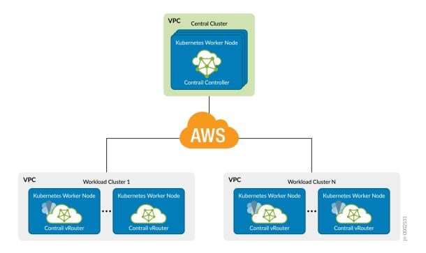
Centralizing the networking in this way makes the networking easier to configure and manage and easier to apply consistent network policy and security.
