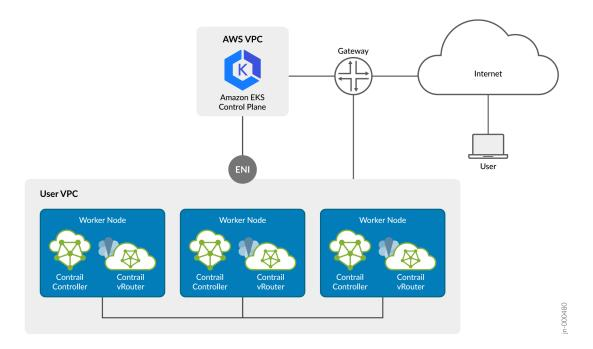
The procedures in this section show basic examples of how you can use the provided Amazon EKS blueprints, Helm charts, and YAML manifests to install CN2 on an Amazon EKS cluster. We cover both installing CN2 in a brand new cluster and in an existing cluster.
