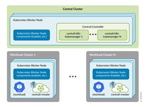
The multi-cluster Contrail controller differs from the single-cluster Contrail controller in two main ways:
