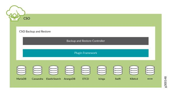
Figure 1 on page 17 shows a conceptual image of how backup and restore is implemented in CSO 4.1. The database systems that are currently backed up within the framework are: MariaDB, Cassandra, ElasticSearch, ArangoDB, Zookeeper, and ETCD. The system also backs up encrypted passwords, and system certificates so that restoring data from any specific backup puts CSO back into the state it was in at the time of that backup.
