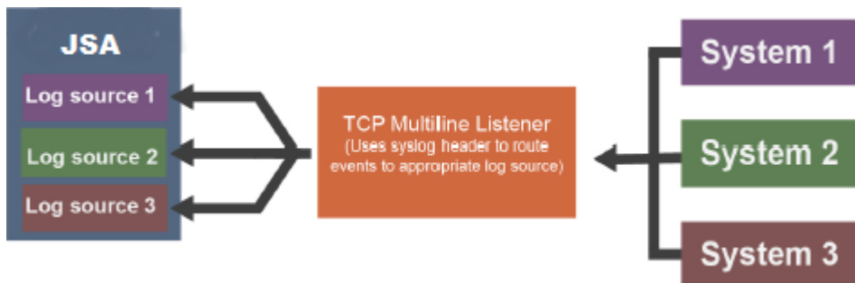
Figure 2: Separate JSA Log Sources Collect Events Sent from Multiple Systems to a TCP Multiline Listener, by Using the Syslog Header.
