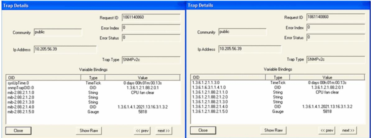
When the CPU fan speed is less than the configured threshold (minimum fan speed), the trap shown in [Figure 49 on page 1025](#) is generated:
