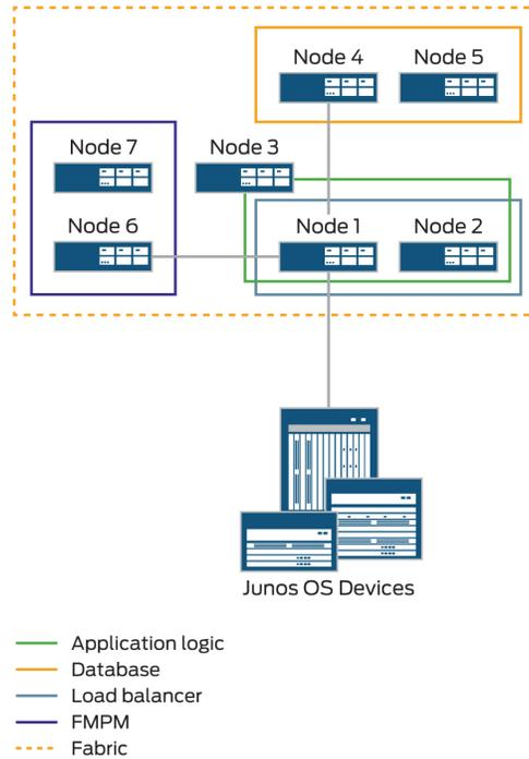
When you add the FMPM node to the fabric, the network monitoring functionality is disabled on the Junos Space nodes and is enabled on the FMPM node. All the devices and nodes now send their traps to the newly added FMPM node. This feature provides you with a high performance network monitoring solution for networks with more than 15,000 small devices or a few devices with thousands of interfaces.
