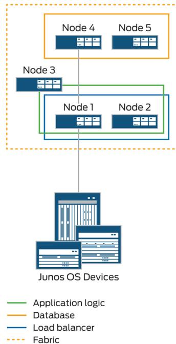
In case the primary database node goes down or is deleted, the database VIP address is transferred to the secondary node, which becomes the new primary database node, and any other non-load-balancer node in the fabric can be designated the new secondary database node. If the secondary database node goes down or is deleted, the primary database node retains the database VIP address and you can designate any other non-load-balancer node as the new secondary database node. If there is no other
