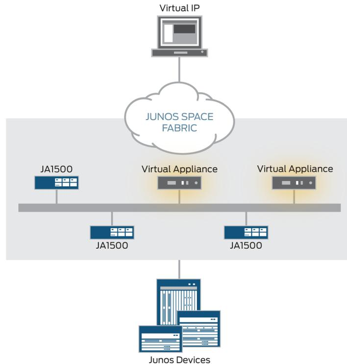
**NOTE:** All nodes that are part of a fabric must have the same version of Junos Space Platform installed.
