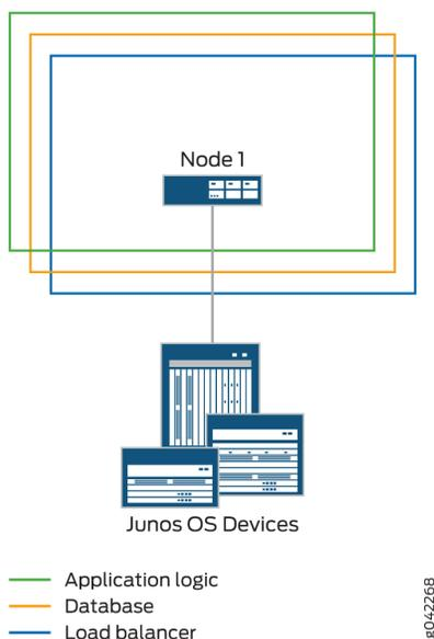
**NOTE:** A fabric that comprises a single node provides no workload balancing and no backup if the Junos Space node goes down.
