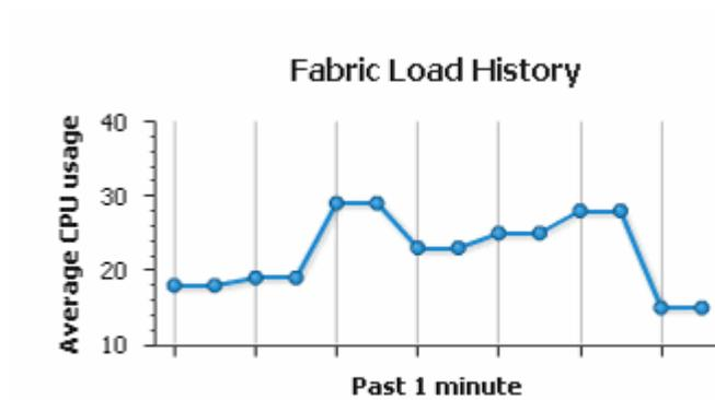
Junos Space Platform uses the following formula to determine the fabric load:  $\text{Fabric Load} = (\text{Total CPU Usage for All Nodes Running}) / (\text{Number of Nodes Running})$
