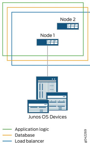
Typically, if the fabric has three or more Junos Space Nodes, only the application logic functionality is enabled from the third node onward. The application logic functionality provides both scalability and high availability. However, high availability for application logic is not available if both the first and second nodes are down. For high availability of application logic, at least one among the first and second nodes should be up.
