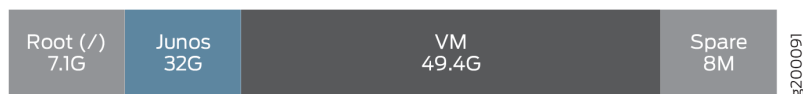
Figure 15: Host partition table for Routing Engines on MX2010 and MX2020 routers with 100GB SSD
