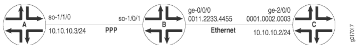
Figure 133: Sample Topology of Layer 2.5 Translational Cross-Connect
