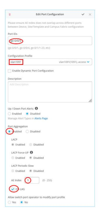
On the switch between the fabric and the DHCP server, you add a simple LAG configuration such as the one below:
