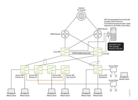
Figure 1: EVPN Multihoming with 2 Collapsed Cores
