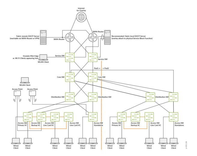
Figure 4: 5-Stage IP Clos, Service Blocks and PoDs
