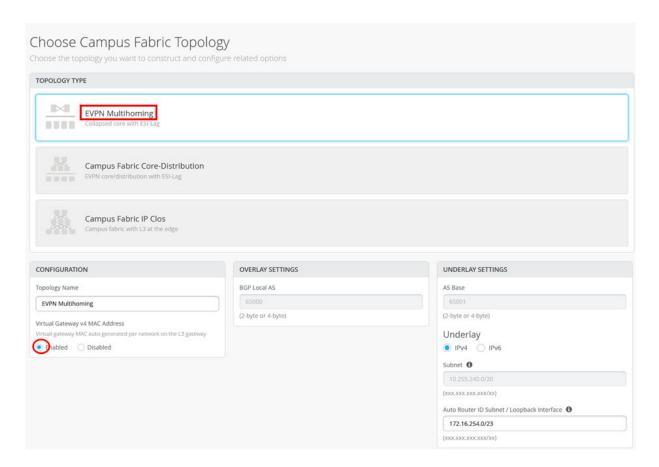
Assign the switches as collapsed cores and access switches in the next pane.
