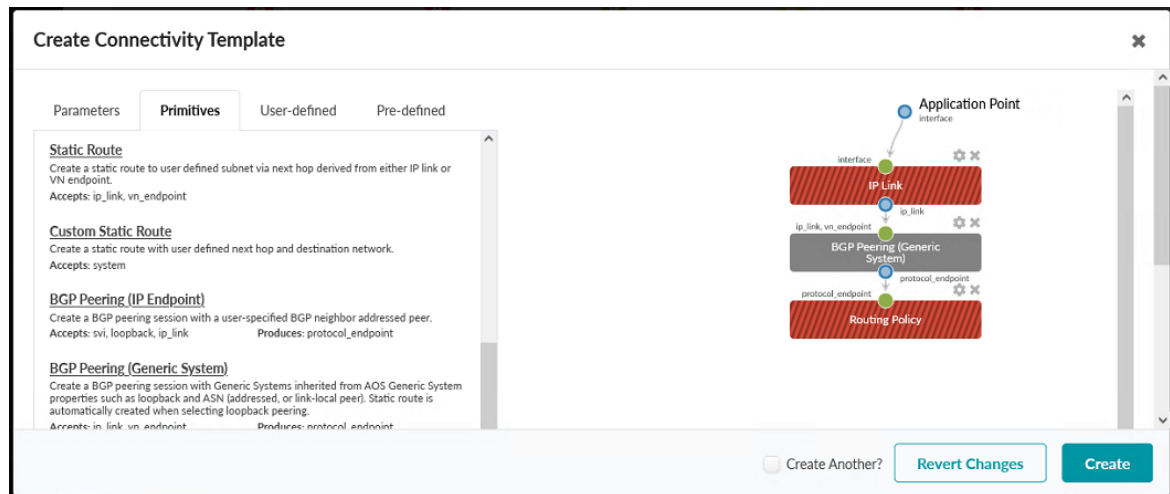
Figure 57: Primitives Tab in the Create Connectivity Template Pop-up in the JVD_CF_without-Access_BluePrint_SM Blueprint
