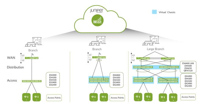
The design of the WAN router can be either redundant or not, depending on customer requirements. Typically, the WAN router at a branch serves as the termination point for the Layer 2 VLANs used by wired switches and attached access points, acting as the default gateway for these devices. Additionally, the WAN router is expected to handle DHCP lease management, either by implementing a DHCP server or by acting as a DHCP relay.
