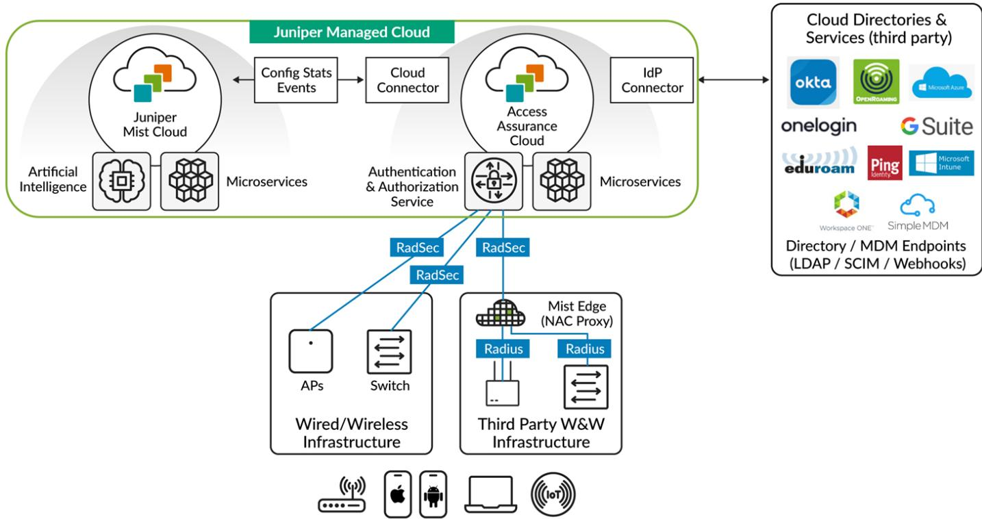
This JVD focuses on all aspects of the Access Assurance offering where the cloud-based Mist Authentication service provides authentication and policy decision making for Wireless or Wired Client independent if they are associated to a Juniper switch, Access Point or to a third-party. The JVD explains the most common deployment scenarios and topologies used. The JVD contains information about the tests operated for these typical deployments as well as best practices.
