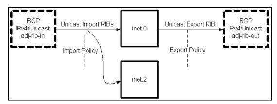
Additionally, RIB groups are useful when using multiprotocol BGP (MBGP). MBGP has the capability of tagging routes as belonging to different virtual topologies. The following configuration specifies MBGP routes tagged as unicast routes to be imported to and exported from inet.0, while routes tagged as multicast routes are imported to and exported from inet.2.
