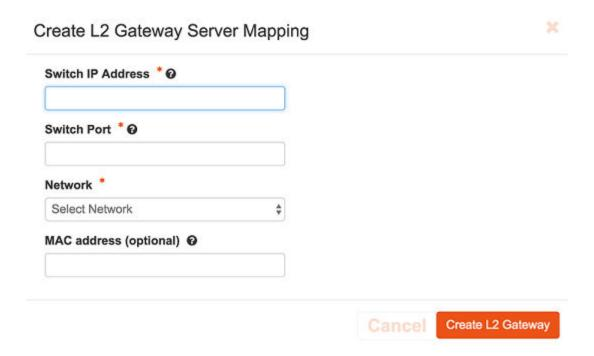
Users can create an L2 Gateway by specifying the switch IP address, wherein the switch must be present in the topology, the interface connecting the BMS, the OpenStack network to be connected to, and optionally the BMS MAC address (required for dhcp to allocate IP address).
