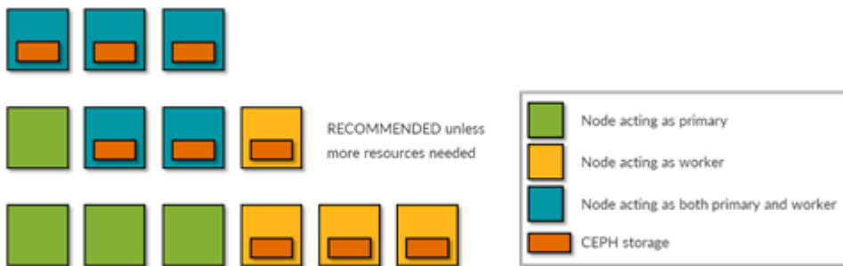
Figure 10: Multinode Redundant Setups
